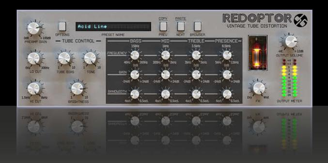
equalizer section will further process the tone of your signal. It allows you to tweak the Frequency, Gain and Bandwidth (Q). d16 states that most typical amps available have a fixed graphical equalizer, with 3 or 4 bands and only allow gain of the signal. With Redoptor's EQ, the bands are controllable making it more flexible and unique.
